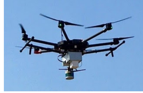
Fig. 2. Our sUAS is a DJI Matrice M600 that carries a LAMP sensor. In the image, the LAMP system can be seen underneath the sUAS and includes a LiDAR puck. The attached white box contains the radiation detection or imaging instrument.
